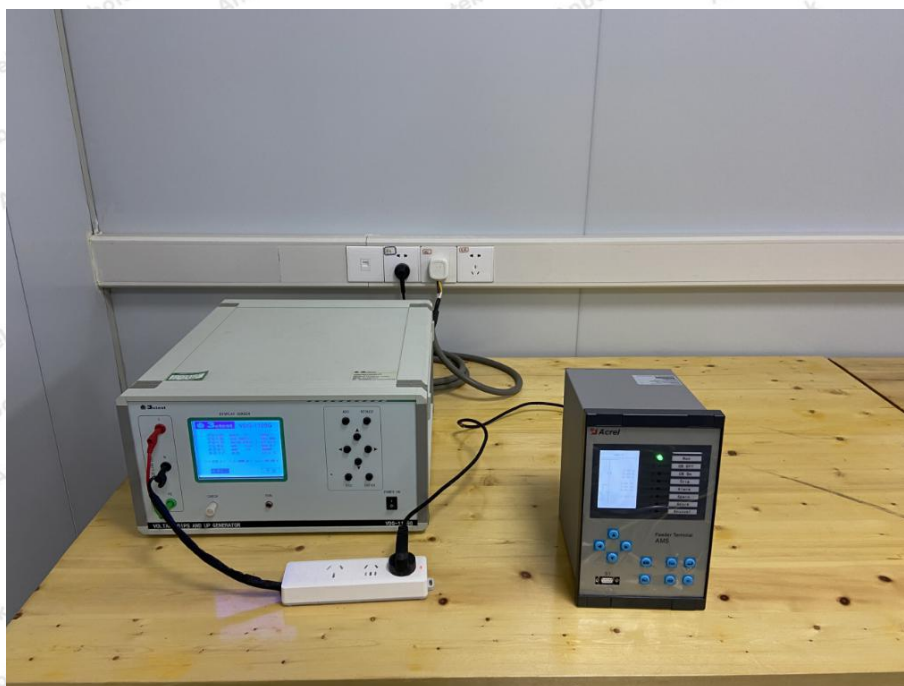
Photo of Voltage Dips and Interruptions Test
