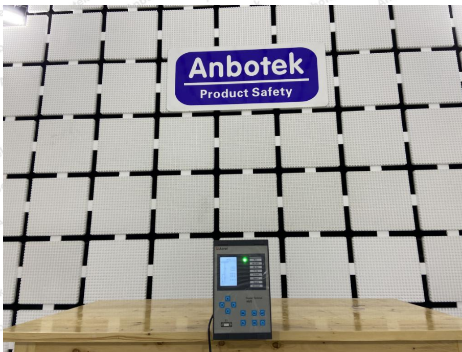
Photo of RF Field Strength susceptibility Test
