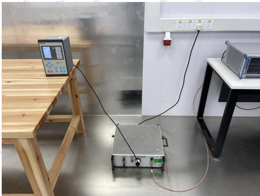
Photo of Power Line Conducted Emission Test
