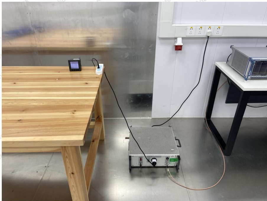
Photo of Power Line Conducted Emission Test
