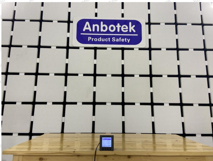
Photo of RF Field Strength susceptibility Test
